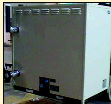
Figure 6: The left photo shows a 260-ton (914 kW) waste-heat-fired absorption refrigeration unit that provides -25^{\circ}\text{C} ( -13^{\circ}\text{F} ) chilling at an oil refinery. The ammonia water air conditioner, shown at right, is designed for microturbine waste heat operation.
