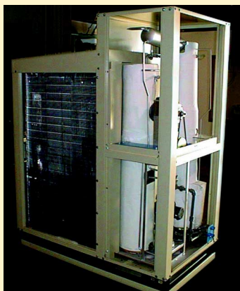
Figure 5: Five-ton (18 kW) gas air conditioner in development.
