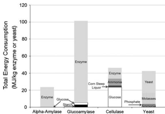
**Fig. 1** Contribution of ingredients and manufacturing to the energy consumption (MJ/kg) during enzymes and yeast production (Note renewable energy contained in bio-derived compounds (e.g., corn starch) not included)
